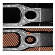
Using a set of 9 cameras, images are taken from various angles for a precision cast part used in the automotive industry. These images are then analyzed for anomalies using Machine Vision and Deep Learning algorithms to identify any surface anomalies. Using this system is very easy and and multiple variants can be inspected with a single setup.
