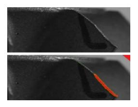
Using a front facing camera, images taken on turbine blades can find chips, dents and scratches of critical nature which are very hard to observe with the naked eye. Using a combination of Artificial Intelligence as well as Machine Vision techniques, reliable detection can be performed.
